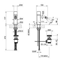
Bidet mixer with waste and connecting flexibles. INTRECCIO
