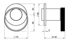
External parts wall-mounted basin separate control, one-way
