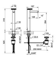
Basin mixer high, short spout, flexible connections, with waste
