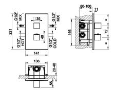
External parts for thermostatic mixer, two-way diverter
