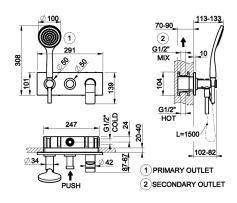
External parts for two-way built-in shower mixer with automatic diverter, water outlet, handshower hook, flexible hose and antilimestone handshower
