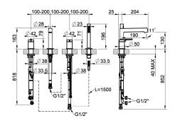
Four-holes bath mixer with diverter, tub-filler spout and 1,50 m flexible hose and antilimestone handshower
