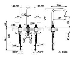
Medium version three-hole basin mixer, with flexible hoses. Without waste
