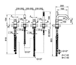
Four-holes bath mixer with diverter, tub-filler spout and 1,50 m flexible hose and antilimestone handshower
