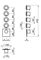
External parts for wall-mounted thermostatic high-capacity mixer. Vertical/horizontal setting up with FOUR SEPARATE EXITS
