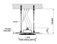
350X350 multifunction system for false-ceiling installation. With RAINFALL/WATERFALL/MIST function. To be completed with cover
