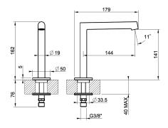
Deck-mounted washbasin spout only without pop-up assembly • Spout projection 5-11/16" • Height 6-3/8"• 1/2" connections• Drain not included - See DRAINS section• Requires handle kit • Max flow rate 1.2 GPM
