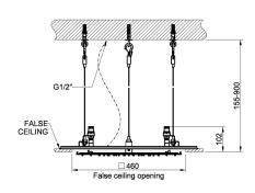
500X500 shower system for false-ceiling installation. With RAINFALL function. To be completed with cover
