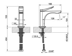
Basin mixer, flexible connections, without waste. Ø25 mm cartridge
