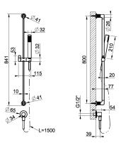
Sliding rail with antilimestone handshower, 1,50 m flexible hose and water outlet
