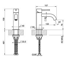
Single lever washbasin mixer without pop-up assembly• Spout projection 4-13/16"• Height 6-1/4"• Drain not included - See DRAINS section• Max flow rate 1.2 GPM• ADA compliant• Handle kit
