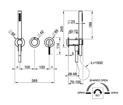
TRIM PARTS ONLY. Wall-mounted bath mixer control• Separate backplate• Two-way diverter• Water outlet• Handshower max flow rate1.75 GPM• Requires inline Pressure Balance
