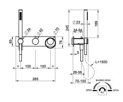
TRIM PARTS ONLY. Wall-mounted bath mixer control Single backplate Two-way diverter Water outlet Handshower max flow rate 1.75 GPM Requires inline Pressure Balance
