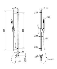
Sliding rail with water outlet, antilimestone handshower and 1,50 m flexible hose.
