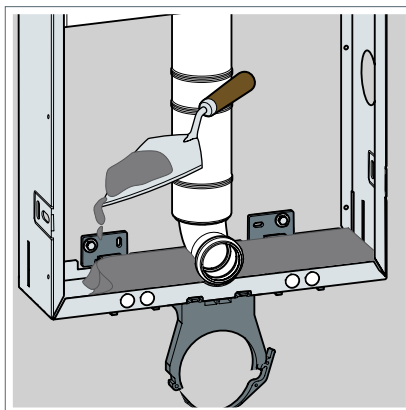
Fig. 50: Filling up the floor of the WC block with mortar.
