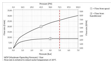
The indicated flow rate values are the result of theoretical measurements conducted using certified laboratory instruments
