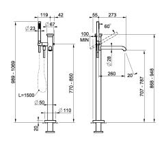
External part for freestanding external bath mixer with hand shower, automatic diverter and Cromalux flexible hose. Can be combined with inserts with different finishes: art. 66600 and art. 66602.
