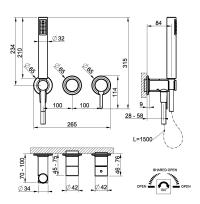
External parts wall-mounted for shower mixer, two way with diverter, water outlet, handshower hook.
