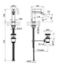
Bidet mixer with waste and connecting flexibles. RIGATO.
