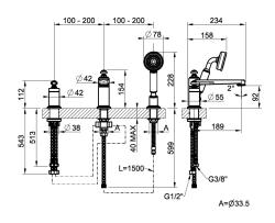
Three-hole basin mixer with diverter, spout, 1,50 m flexible hose and pull-out antilimestone handshower
