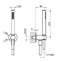
Handshower set • Fixed hook • Wall elbow • 59" flex hose • Max flow rate 1.75 GPM
