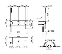
External parts wall-mounted for shower mixer, two-way, diverter, water outlet, handshower hook
