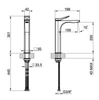
High basin mixer, flexible connections, without waste. Ø35 mm cartridge
