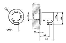
Wall elbow with backplate • 1/2" connection
