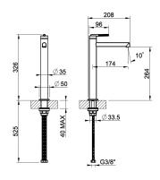
Tall single lever washbasin mixer without pop-up assembly• Spout projection 6-7/8"" • Height 12-13/16" • Drain not included - See DRAINS section • Max flow rate 1.2 GPM • ADA compliant
