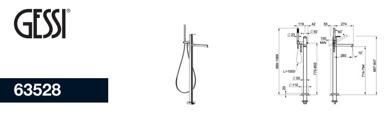
TRIM PARTS ONLY floor-mounted tub filler • Handshower • 59" flex hose • diverter • Spout projection 10-1/4" • Handshower max flow rate 1.75 GPM • Spout mixed flow rate 6 GPM at 60 PSI • Requires in-floor rough valve 48189
