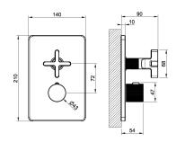
External parts for thermostatic mixer, two-way diverter
