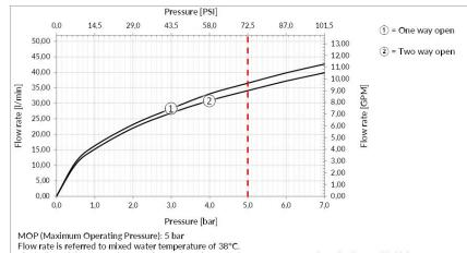
The indicated flow rate values are the result of theoretical measurements conducted using certified laboratory
