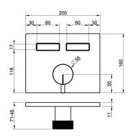
External parts for single-lever mixer for two separate functions, with push-button on/off controls.
