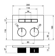
TRIM PARTS ONLY External parts for thermostatic mixer for three functions, with push-button on/off control• Single backplate• 1/2"connections• Anti-scalding• Requires in-wall rough valve 63001• Non-Shared function
