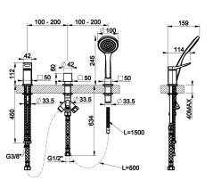
Three-holes bath mixer with diverter, 1,50 m flexible hose and antilimestone handshower. To be used with overflow filler
