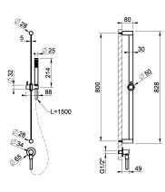
Handshower and adjustable sliding rail set● Adjustable bar● Adjustable hook● 59" flex hose● Wall elbow● Max flow rate 1.75 GPM
