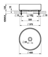
Counter washbasin Ø400mm in stainless steel, without overflow waste. Without basin waste. It can be combined with waste 54599.
