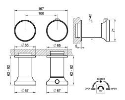
External part wall-mounted thermostatic two-ways shower mixer. Can be combined with inserts with different finishes: art. 66600 and art. 66602.
