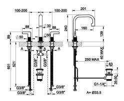
Medium version three-holes basin mixer, with flexible hoses with waste
