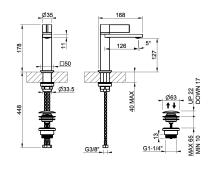
Basin mixer with Stop&Go waste and connecting flexibles. DIAMANTATO.
