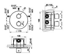
External parts for thermostatic mixer, three-way diverter
