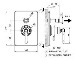
External part wall-mounted mixer, two-way automatic diverter
