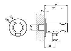
Wall elbow with built in water intake and fixed hook● 1/2" connection
