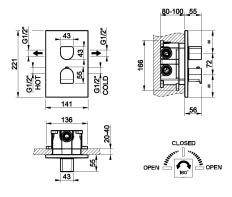
External parts for thermostatic mixer, two-way diverter
