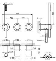
External parts wall-mounted two-way shower mixer with diverter, water outlet, hand shower hook and hand shower.
