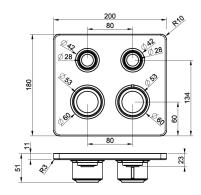
TRIM PARTS ONLY External parts for thermostatic mixer for two functions, with push-button on/off control Single backplate 1/2" connections Anti-scalding Requires in-wall rough valve 63001 Non-Shared Function
