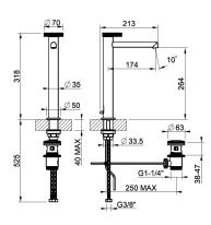
High version basin mixer, long spout, flexible connections, with waste
