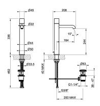
High version basin mixer with waste and connecting flexibles. RIGATO
