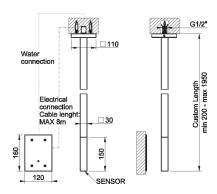
External part for Ceiling-mounted Electronic mixer, lenght on request, with temperature and water flow rate adjustment through under-basin control (included)
