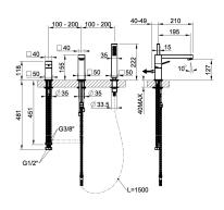
Three-holes bath mixer with diverter in the spout, 1,50 m flexible hose and antilimestone handshower
