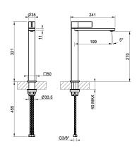
High version basin mixer without waste, with connecting flexibles. RIGATO.
