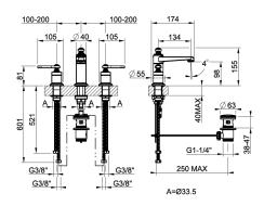
Medium three-hole basin mixer, with flexible hoses, with waste
